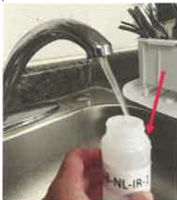
Figure 4. Photo of sample collection process. Arrow indicates neck of the bottle where the bottle should be filled to.
